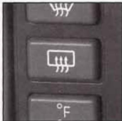
The lines you see on the rear window warm the glass. Press the button to start warming your window. If you have the standard system, a light will glow in the switch while the defogger is working.
