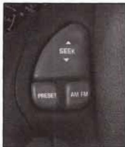
If your vehicle has this feature, you can control certain radio functions using the buttons on your steering wheel.
