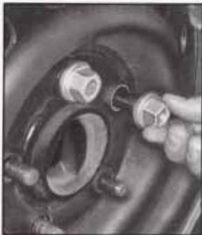
9. Replace the wheel nuts with rounded end of the nuts toward the wheel.
