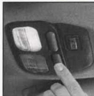
These front reading lamps and the interior courtesy lamps will come on when you open the doors.
