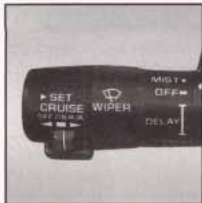
With cruise control, you can maintain a speed of about 25 mph (40 km/h) or more without keeping your foot on the accelerator. This can really help on long trips.
