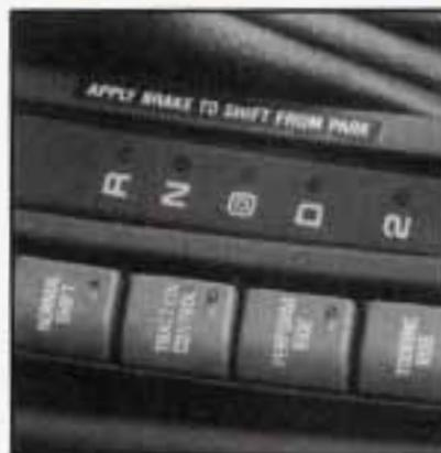
Press **PERFORM SHIFT** to allow the transaxle to shift at higher engine speeds, increasing acceleration performance. An indicator light on the switch will glow when performance shifting is in operation.
