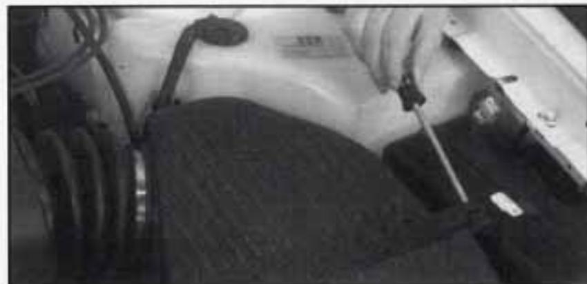
1. Remove the screws on the air cleaner housing cover.
