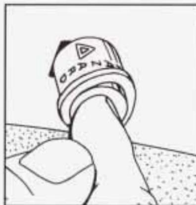
Press the button in to make your front and rear turn signal lamps flash on and off.
