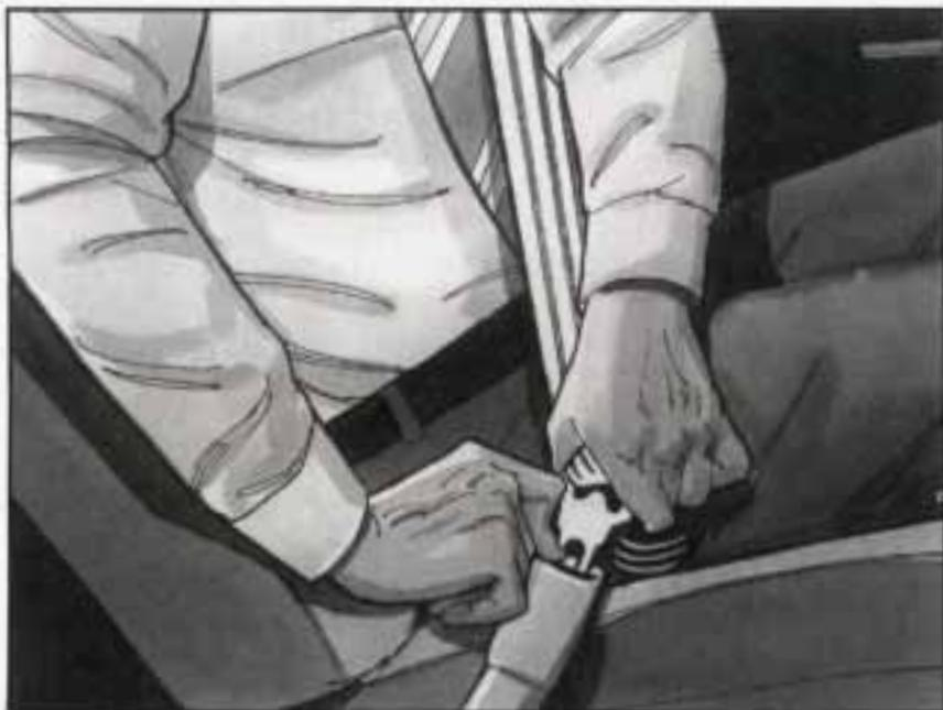
To unclatch the belt, just push the button on the buckle. The belt should go back out of the way.
