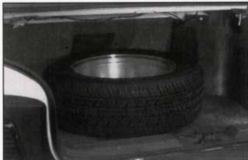
After you've put the compact spare tire on your vehicle, you'll need to store the flat tire in your trunk. Use the following procedure to secure the flat tire in the trunk.
