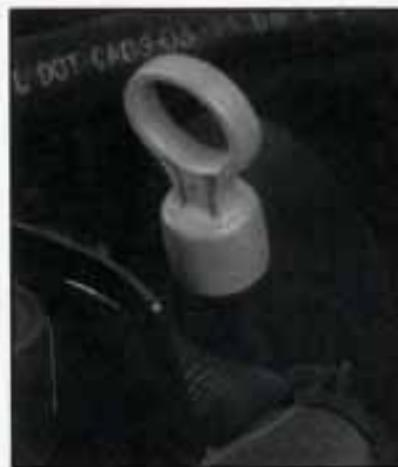
1. The transaxle fluid dipstick top is a round, red loop and is next to the brake master cylinder behind the engine block. Pull out the dipstick and wipe it with a clean rag or paper towel.
