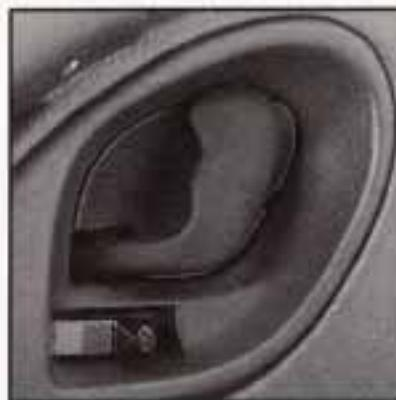
To lock the door from the inside, slide the locking lever rearward. To unlock the door, slide the locking lever forward.
