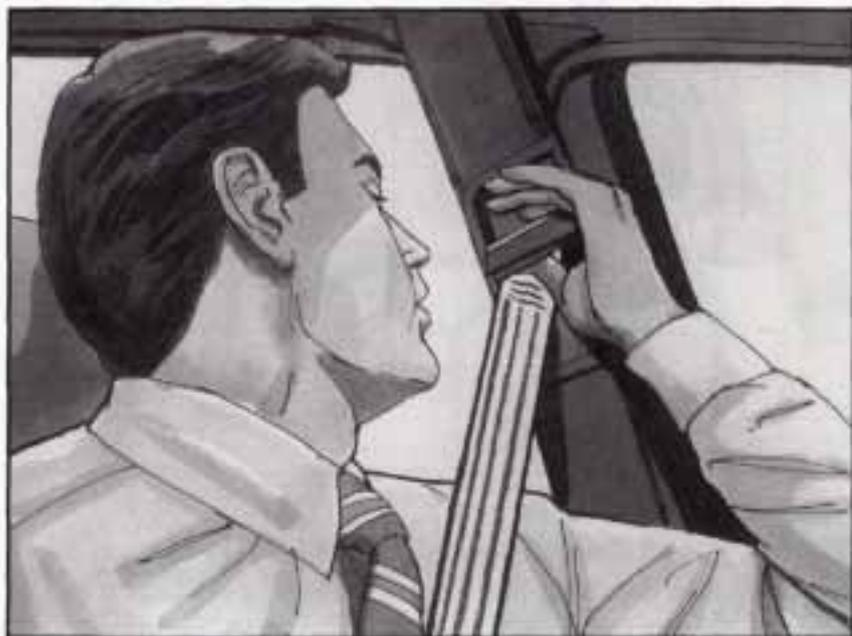
To move it down, squeeze the release handle and move the height adjuster to the desired position. You can move the adjuster up just by pushing up on the bottom of the release handle. After you move the adjuster to where you want it, try to move it down without squeezing the release handle to make sure it has locked into position.
