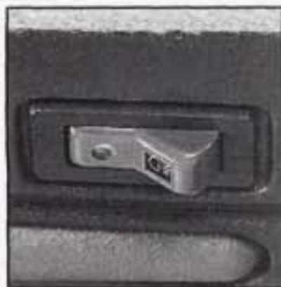
The fog lamps switch is in the front of the front reading lamps.
