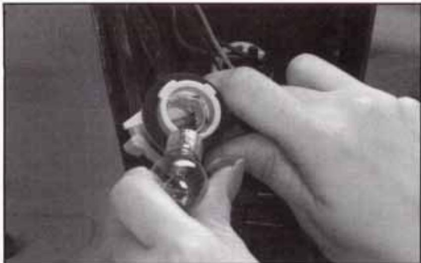
8. If you are replacing the back-up bulb, it must be turned and pulled out to be removed.
