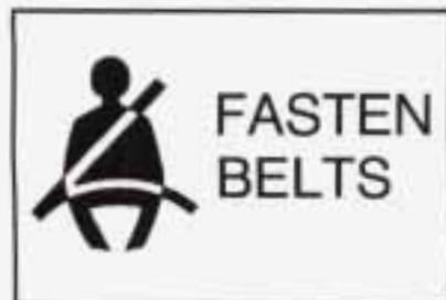
The safety belt light will also come on and stay on for about 70 seconds. If the driver's belt is already buckled, neither the chime nor the light will come on.
