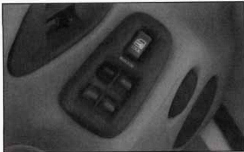
Switches on the driver's door panel control each of the windows when the ignition is on or when retained accessory power is active. In addition, each passenger door has a control switch for its own window.
