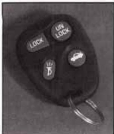
If your vehicle has this option, you can lock and unlock your doors or unlock your trunk from about 3 feet (1 m) up to 30 feet (9 m) away using the remote keyless entry transmitter supplied with your vehicle.
